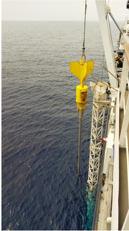
Fig. 8. The gravity core system used in this Campaign (barrel length of 5 m in this photograph).
