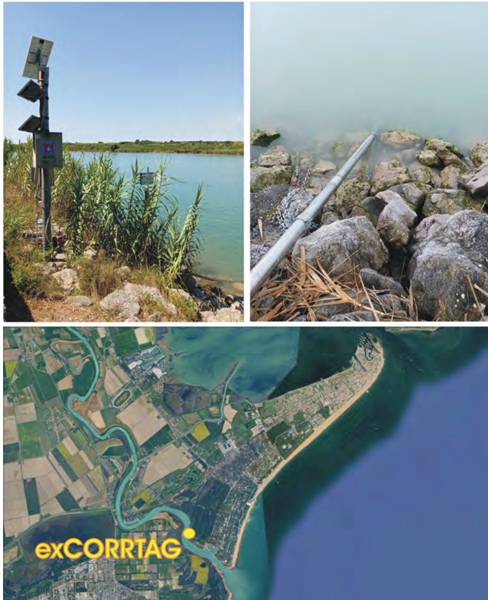
Figure 61 - Station exCORRTAG located at the mouth of Tagliamento River in the Pine Forest “Riviera Nord”. Automated remote station and the stilling pipe containing CTD instruments are also shown.
