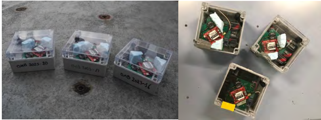
Figure 55 – Example of drifting wave buoys produced by the Norwegian Meteorological Institute (OpenMetBuoys)
