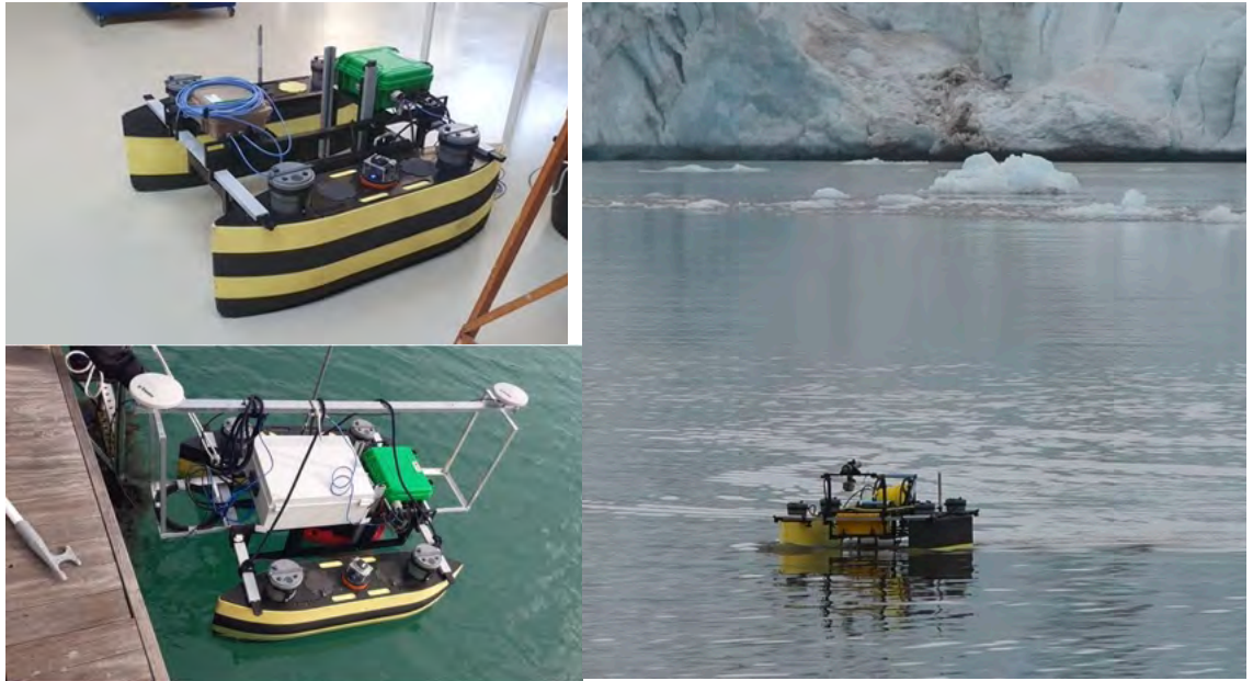
Figure 40 – SWAMP - Shallow Water Autonomous Multipurpose Platform; up left panel) equipped with ROX and SUNA V2; down left panel) equipped with MBES R2- Sonic; right panel) in action in Svalbard Islands
