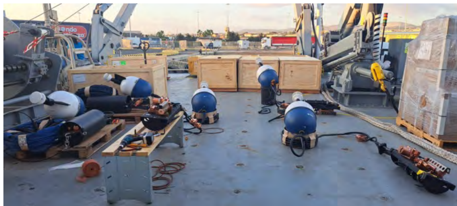
Figure 49 – BGC-SVP drifters on ship deck of R/CV Gaia Blu during the ITINERIS'S EYES cruise.
