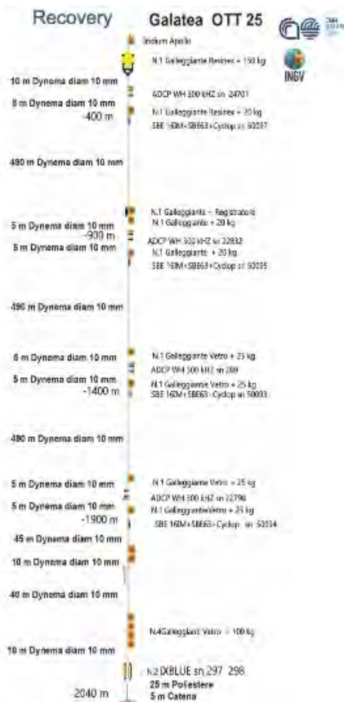
Figure 23 – Galatea Mooring line recovery scheme, October 2025.
