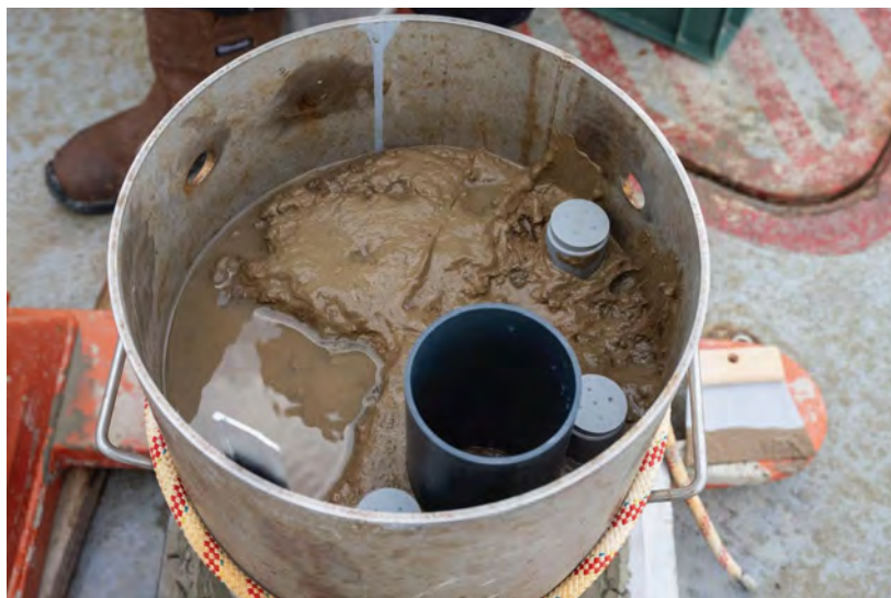
Figure 8.1.9. Liner for stratigraphy and 3 small cores for meiofauna sampling.
