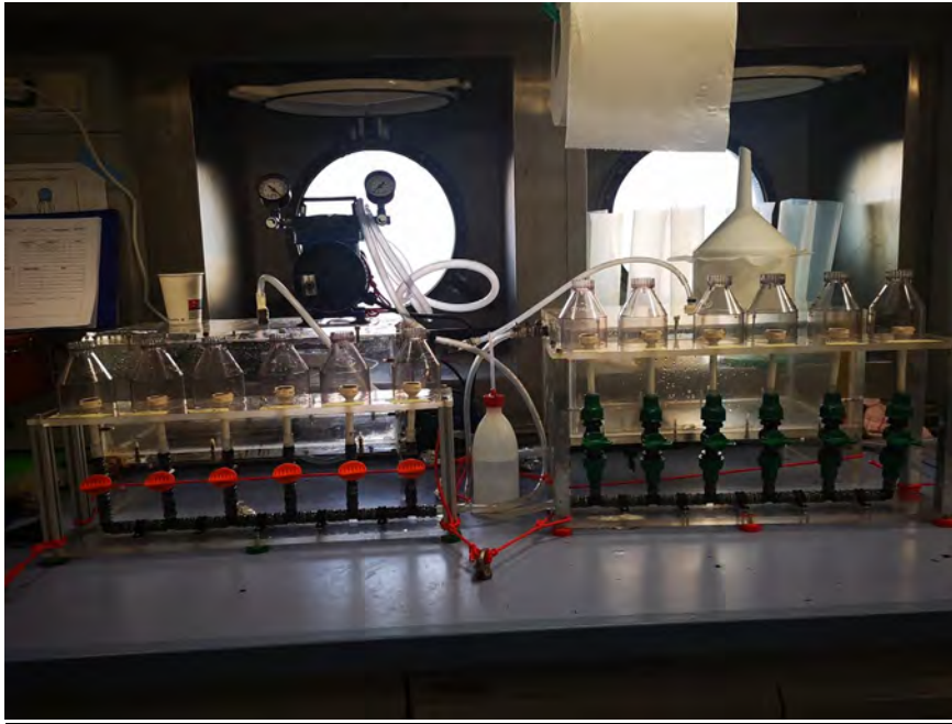
Figure 3.1.5. Filtration apparatus for phytoplankton pigment concentration in the wet lab of the R/V Gaia Blu.
