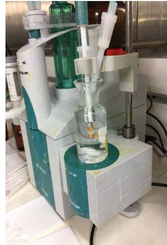
Figure 3.1.1. A. Dissolved oxygen samples (after 2-3 hours storage) and B. the Metrohm Winkler titration instrument used on board for the analysis.
