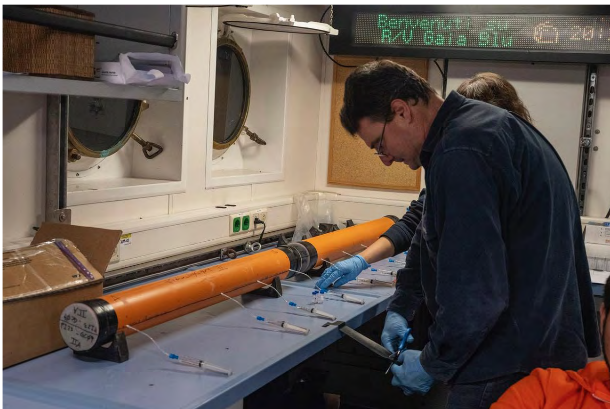
Figure 8.1.6. Pore water sampling performed in the dry lab on board R/V Gaia Blu.
