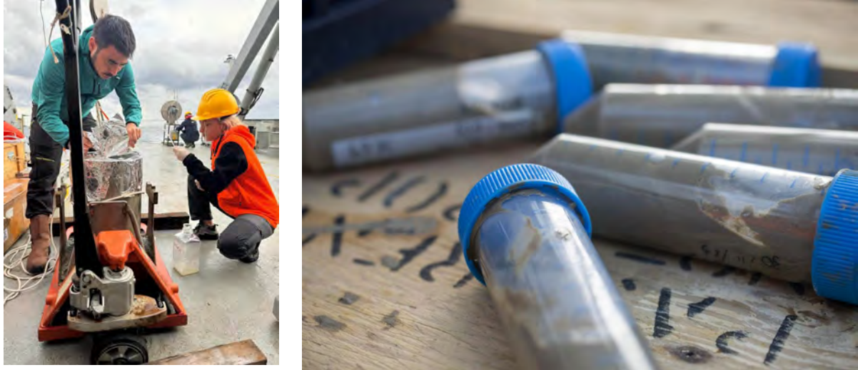
Figure 8.1.8. A. Seawater collection from the box corer and B. falcon tubes filled with sediment.
