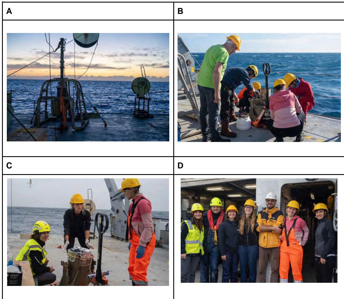
Figure 8.1.7. A. Box corer ready for operations. B. Collection of sediment from outside the cylinder of the box corer for experiments to be conducted on the bulk component. C. Precautionary protection of the sediment from atmospheric input (e.g. microplastics) before sub-sampling D. Box-coring team.
