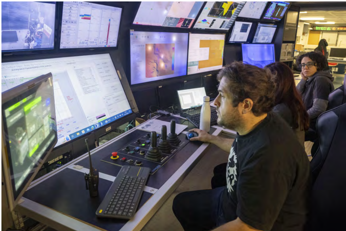
Figure 11.1.1. Remote control of the CTD/Rosette winch from inside the Science Control Room.
