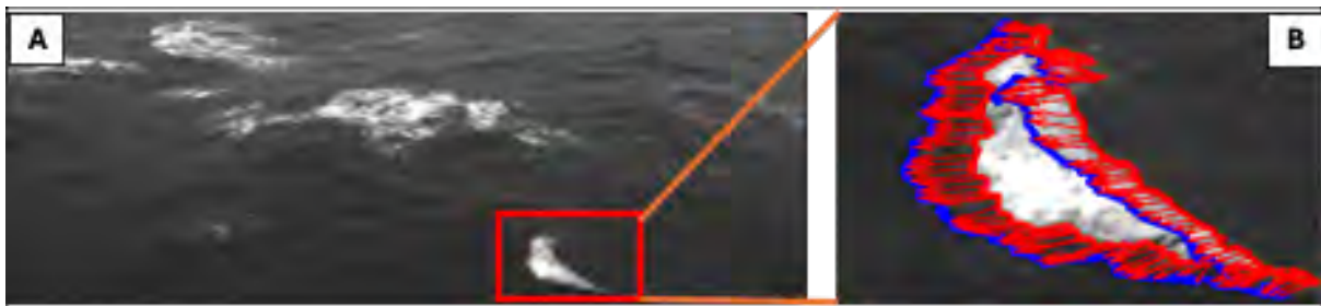
Figure 7 | Panel A shows the sea surface with whitecaps taken from the "Aqua Alta" platform. Panel B shows a closeup of an individually tracked actively breaking whitecap. The arrows represent the movement of the whitecap computed from optical flow image processing technique.
