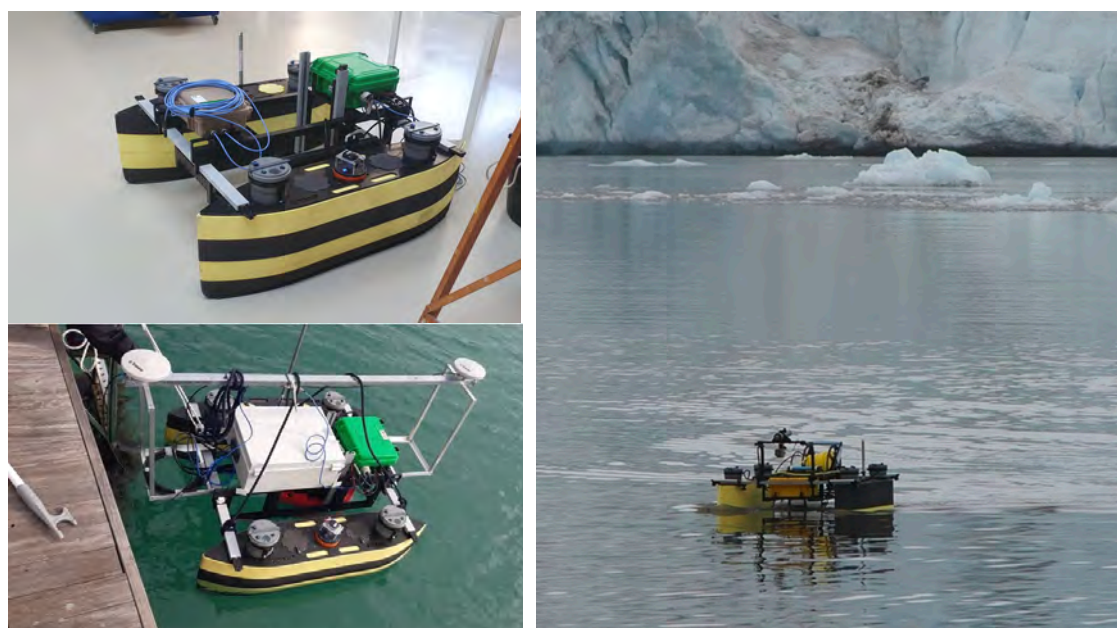
Figure 24 – SWAMP – Shallow Water Autonomous Multipurpose Platform; up left panel) equipped with ROX and SUNA V2; down left panel) equipped with MBES R2– Sonic; right panel) in action in Svalbard Islands
