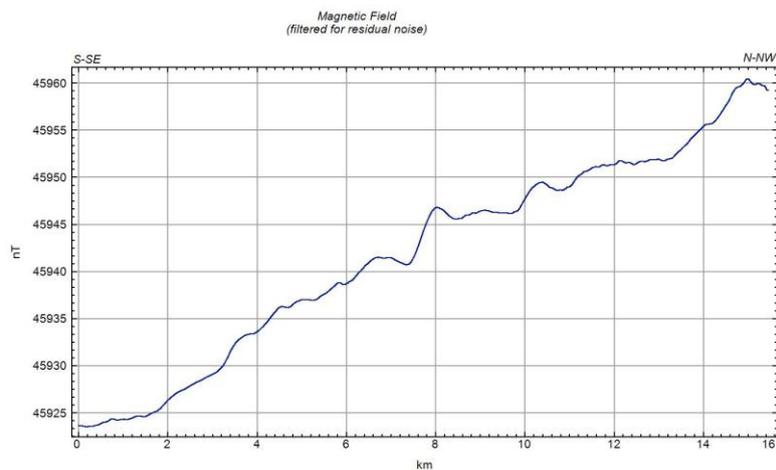
Figure 16. Magnetic field recorded after residual noise removal
