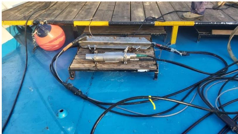
Figure 7 - Seismic source S15 water gun
