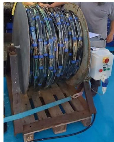
Figure 8 – On left side, air compressor Mod. KA16DD by BAUER. On right side, the receiver system spooled on an electric winch
