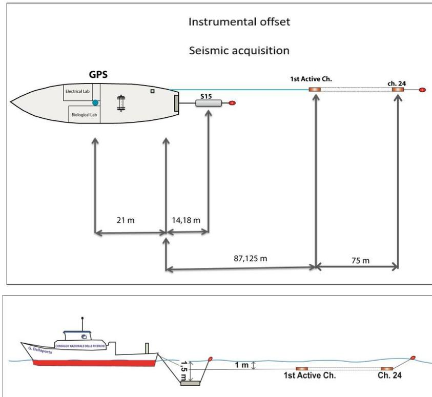
Figure 10 - Offsets of seismic acquisition system towed at the stern of the vessel, plan and side view.
