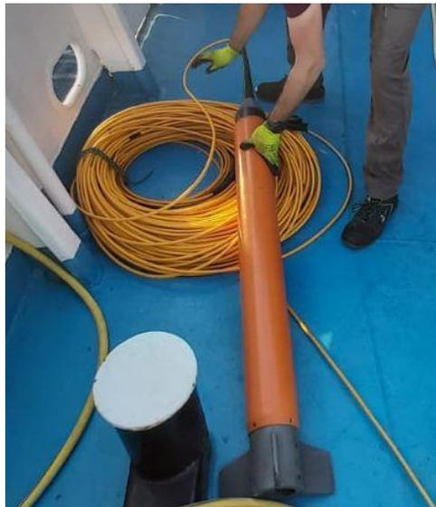
Figure 11 - The SeaSpy magnetometer with the 133 m-length cable
