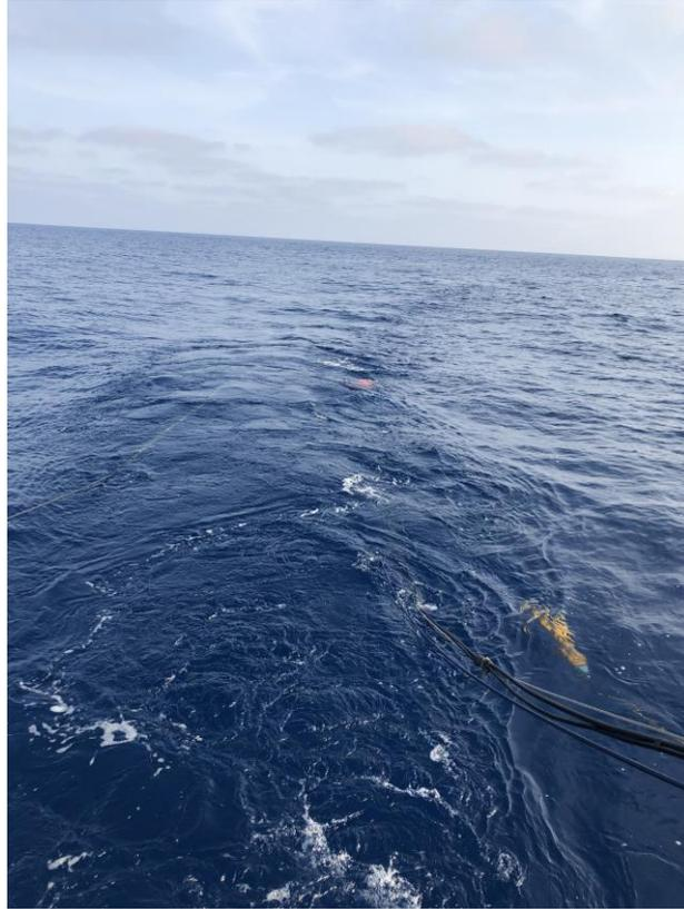
Figure 9 – The photo shows on left the streamer, in the centre the water gun marked also by the presence of the buoy, and on right the magnetometer.
