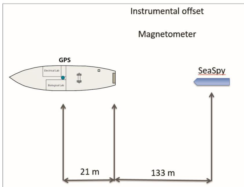
Figure 12 - Off sets of magnetometer towed at the stern of vessel.
