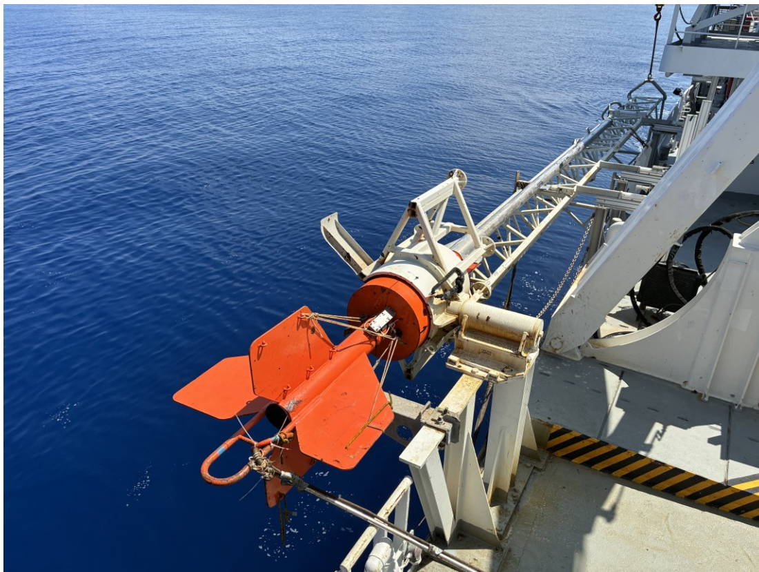
Figure 12 – Photo of Piston Corer system with 5m-long tube, the system is housed in the cradle which allows for safe deployment and recovery of the core barrel.
