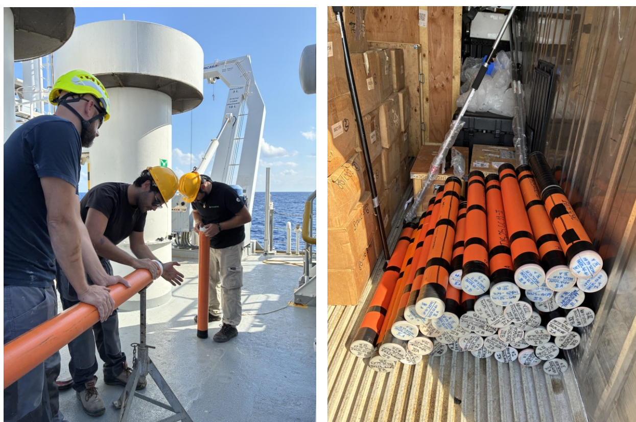
Figure 13 – Sub-sampling of core in 1 m-long section (on left); the core sections stored in refrigerated container.
