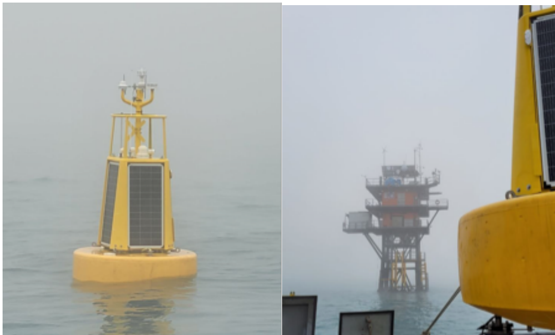
Figure 6 | Deployment of a buoy of the “Italian National Wave Buoy Network” (Rete ondametria Nazionale, RON). (left) The buoy with the floating hull (below, hosting wave and water column characteristics sensors) and its superstructure (above, supporting solar panels and meteorological sensors). (right) The buoy before the deployment. Photo credit: Thomas Pavan.
