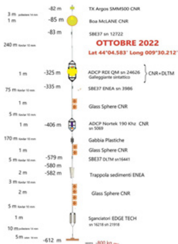
Figure 17– Mooring's structure.
