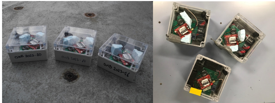
Figure 35 – Example of drifting wave buoys produced by the Norwegian Meteorological Institute (OpenMetBuoys)
