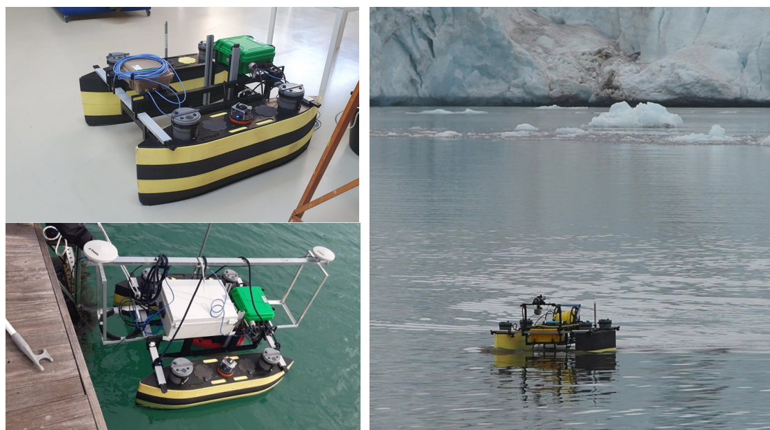
Figure 27 – SWAMP – Shallow Water Autonomous Multipurpose Platform; up left panel) equipped with ROX and SUNA V2; down left panel) equipped with MBES R2– Sonic; right panel) in action in Svalbard Islands
